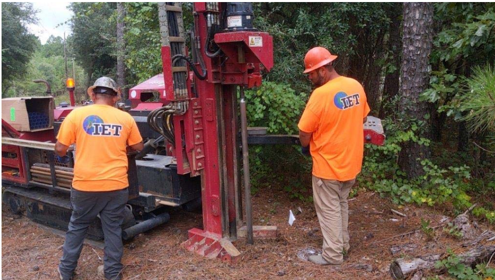
Photograph 6: View of IET advancing direct push soil sampler, photograph taken on different parcel.
