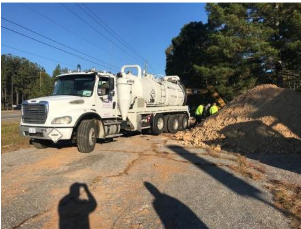
Photograph 1: EVO vacuum truck preparing to extract remaining liquids in USTs.
