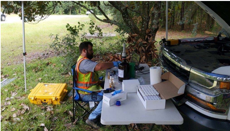
Photograph 8: View of on-Site UVF analysis setup.
