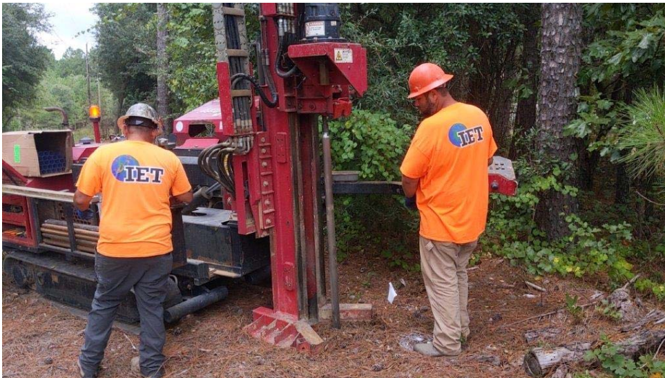
Photograph 6: View of IET advancing direct push soil sampler.
