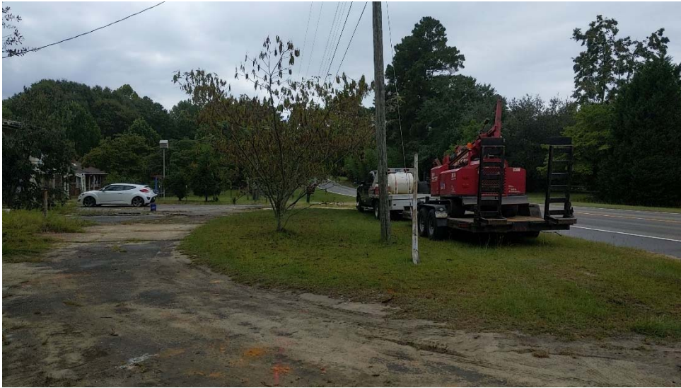
Photograph 7: IET unloading direct-push rig to advance soil borings at parcel 368.
