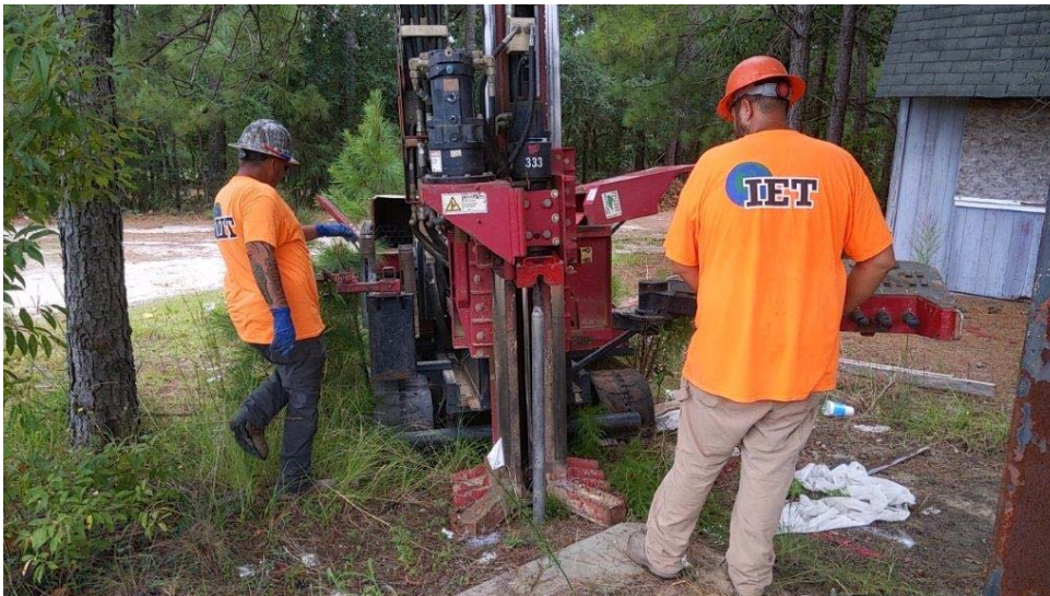
Photograph 4: View of IET advancing direct push soil sampler at parcel 285.
