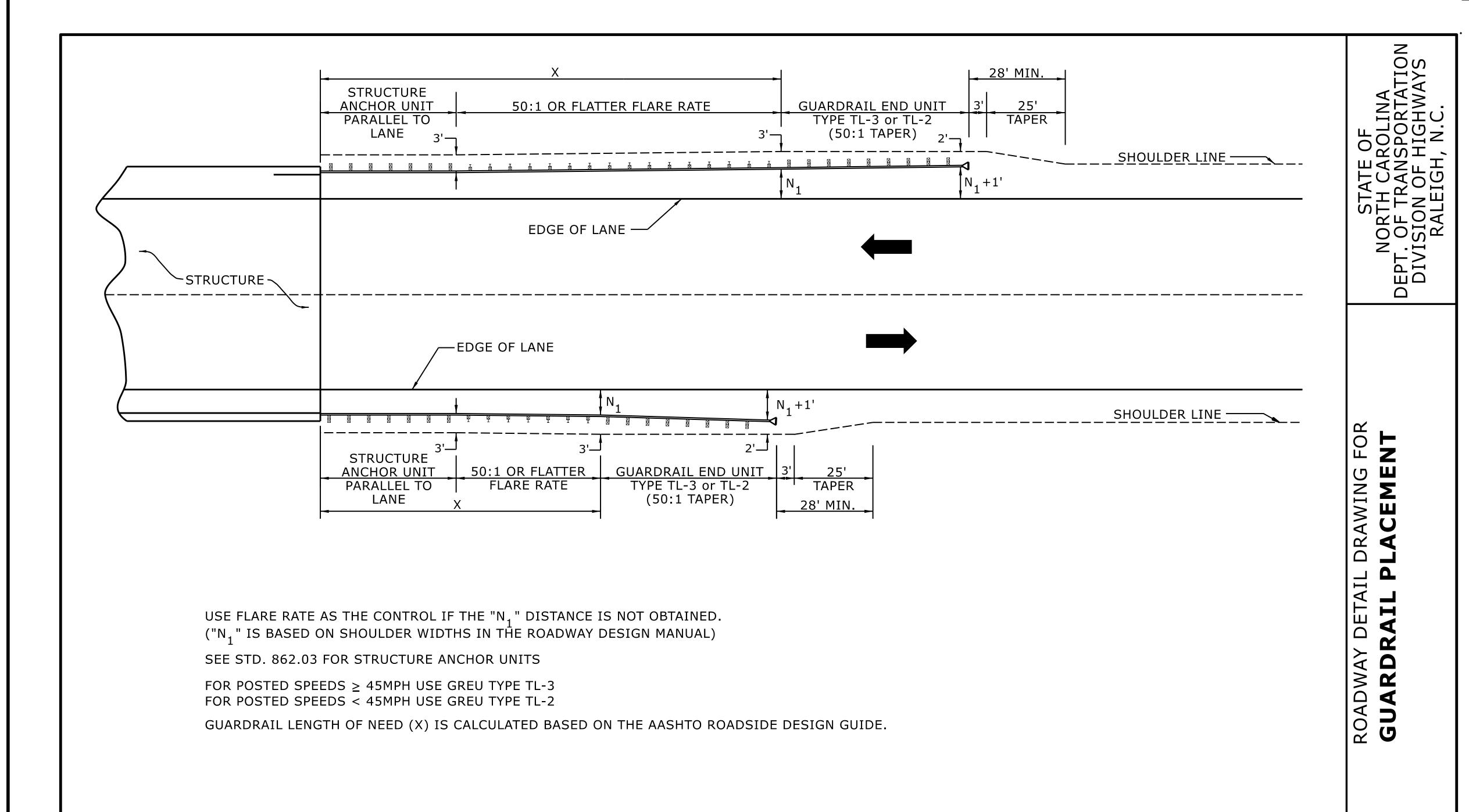
LENGTHS AND OFFSETS FOR PROPOSED GUARDRAIL AT TWO LANE - TWO WAY LOCATIONS
