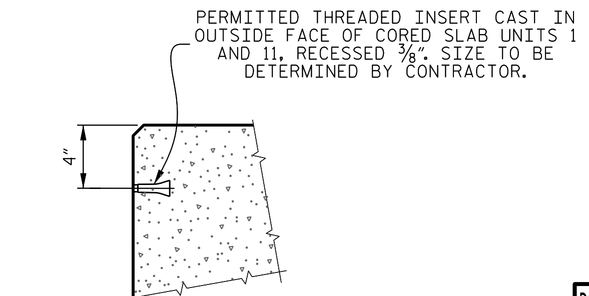
THREADED INSERT DETAIL
