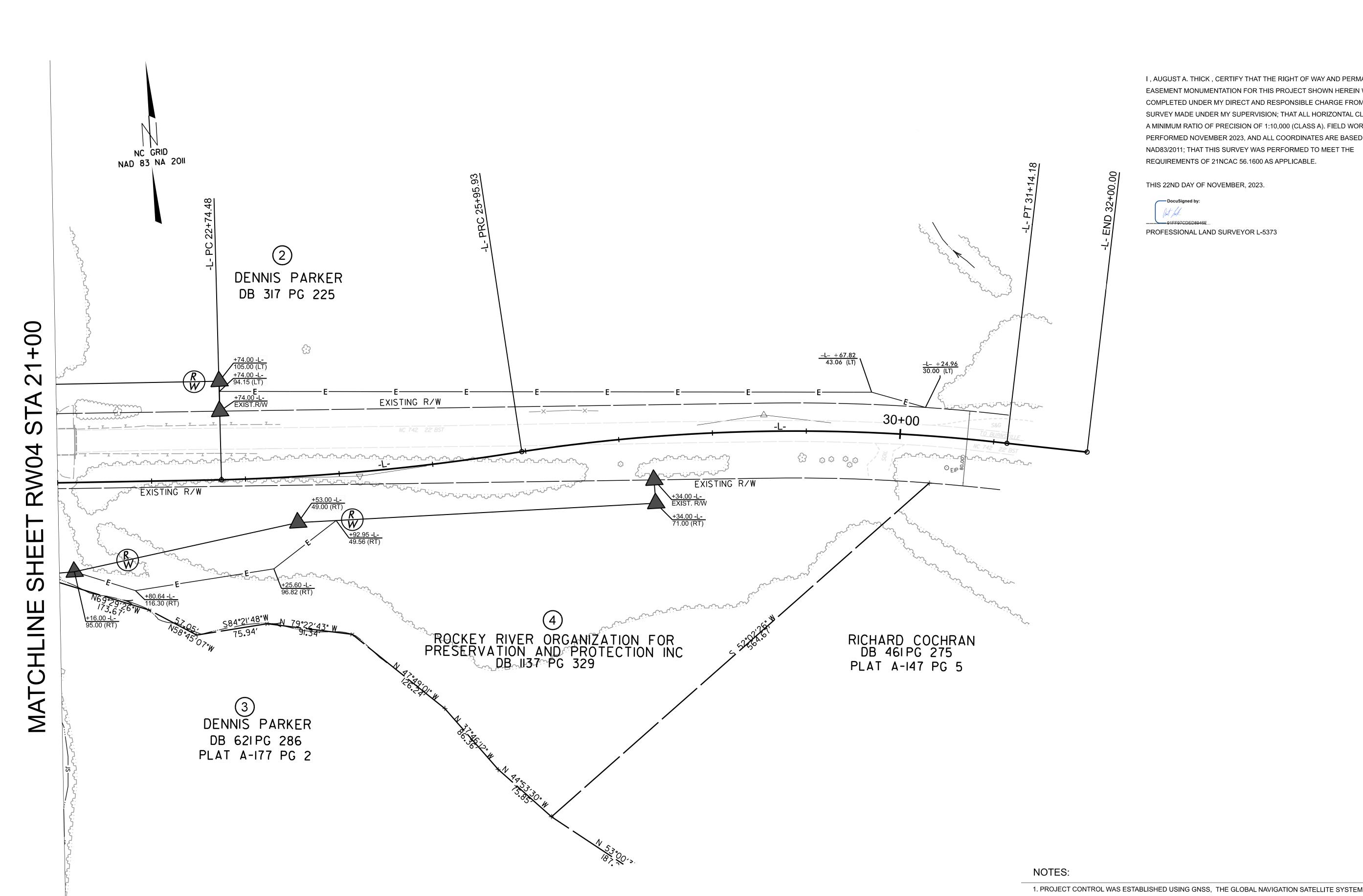
I, AUGUST A. THICK, CERTIFY THAT THE RIGHT OF WAY AND PERMANENT EASEMENT MONUMENTATION FOR THIS PROJECT SHOWN HEREIN WAS COMPLETED UNDER MY DIRECT AND RESPONSIBLE CHARGE FROM AN ACTUAL SURVEY MADE UNDER MY SUPERVISION; THAT ALL HORIZONTAL CLOSURES HAD A MINIMUM RATIO OF PRECISION OF 1:10,000 (CLASS A). FIELD WORK WAS PERFORMED NOVEMBER 2023, AND ALL COORDINATES ARE BASED ON NAD83/2011; THAT THIS SURVEY WAS PERFORMED TO MEET THE REQUIREMENTS OF 21NCAC 56.1600 AS APPLICABLE.
