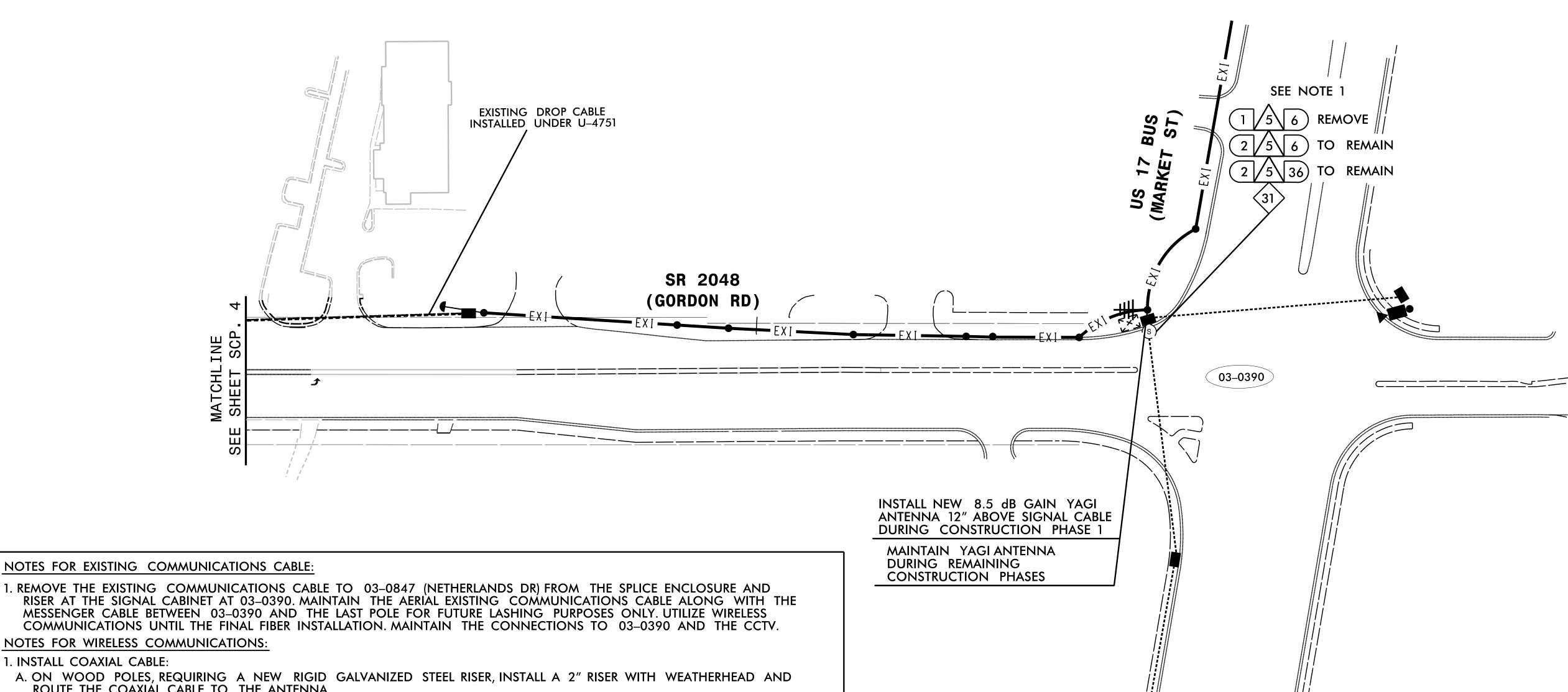
1. REMOVE THE EXISTING COMMUNICATIONS CABLE TO 03-0847 (NETHERLANDS DR) FROM THE SPLICE ENCLOSURE AND RISER AT THE SIGNAL CABINET AT 03-0390. MAINTAIN THE AERIAL EXISTING COMMUNICATIONS CABLE ALONG WITH THE MESSENGER CABLE BETWEEN 03-0390 AND THE LAST POLE FOR FUTURE LASHING PURPOSES ONLY. UTILIZE WIRELESS COMMUNICATIONS UNTIL THE FINAL FIBER INSTALLATION. MAINTAIN THE CONNECTIONS TO 03-0390 AND THE CCTV. NOTES FOR WIRELESS COMMUNICATIONS:
