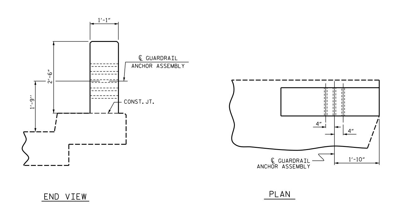
LOCATION OF GUARDRAIL ANCHOR AT END POST
