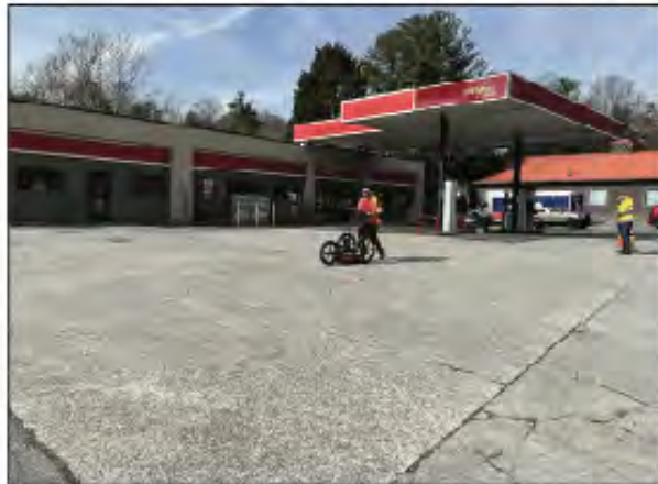
Photo 2. Collecting GPR data at Parcel #019.
