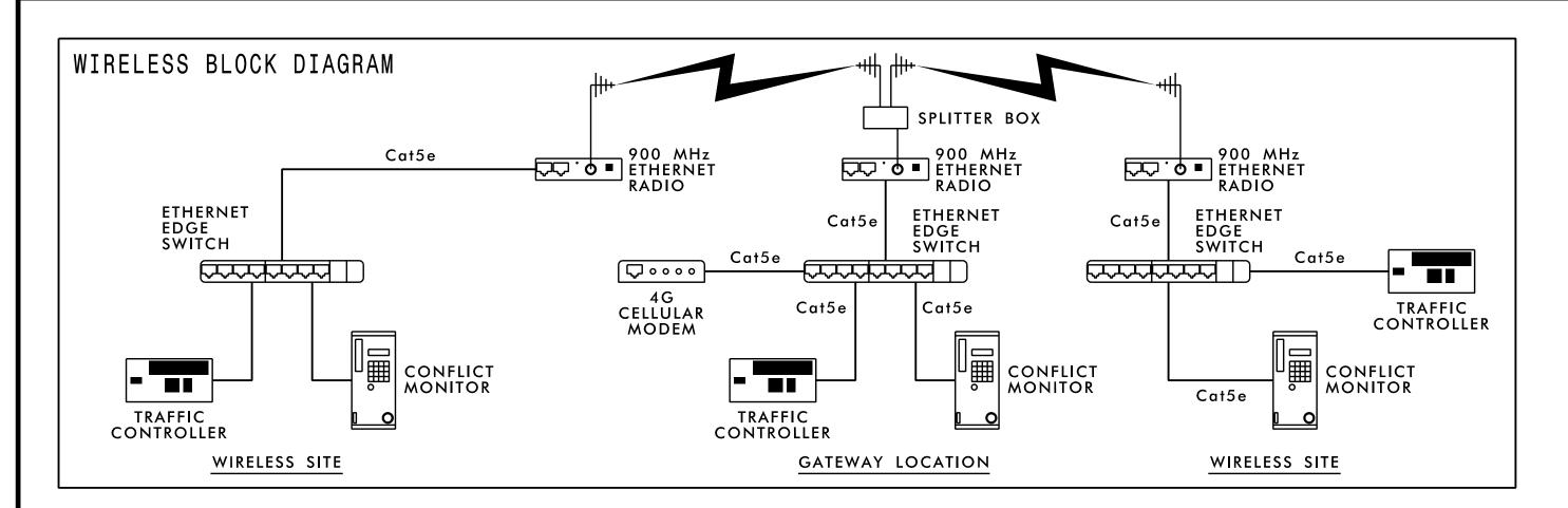
(Cy.) EDGE SWITCH INSTALL 900 MHz ETHERNET RADIO 08-0507 INSTALL 8.5 DB GAIN YAGI ANTENNA ATTACH ANTENNA 12" ABOVE SIGNAL CABLE
