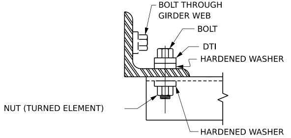
**BOLT WITH DTI ASSEMBLY DETAIL**
