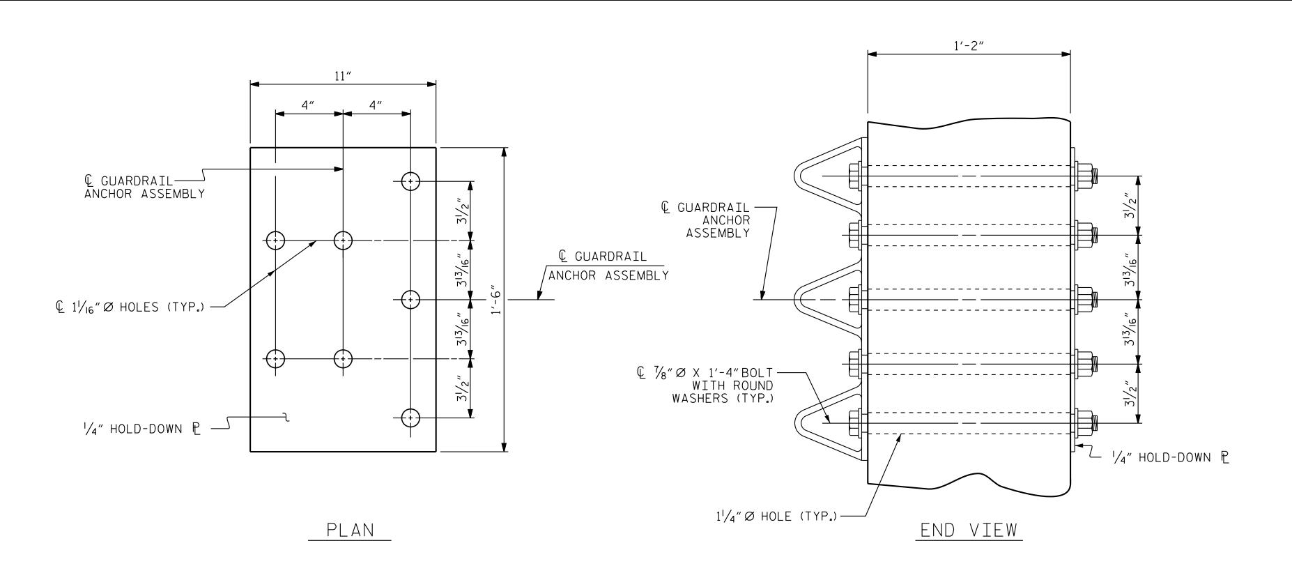
GUARDRAIL ANCHOR ASSEMBLY DETAILS
