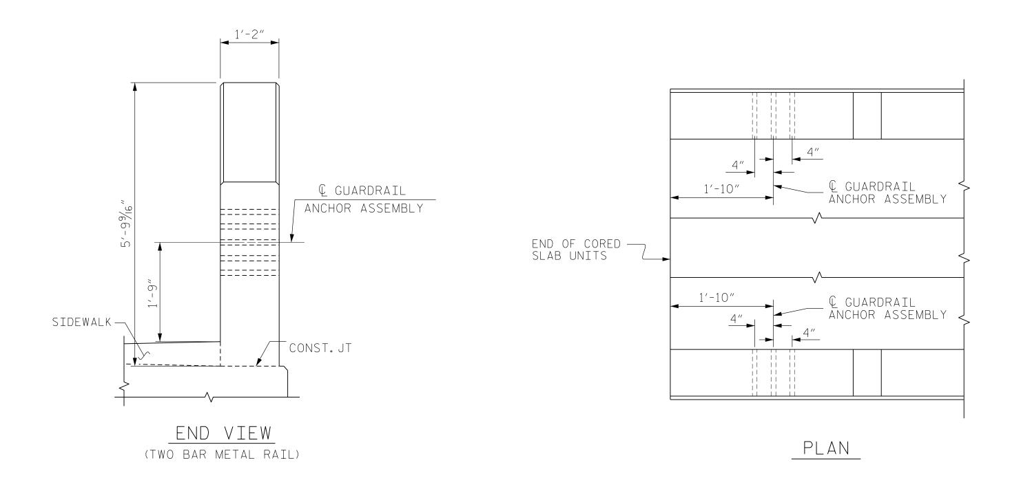
LOCATION OF GUARDRAIL ANCHOR AT END POST
