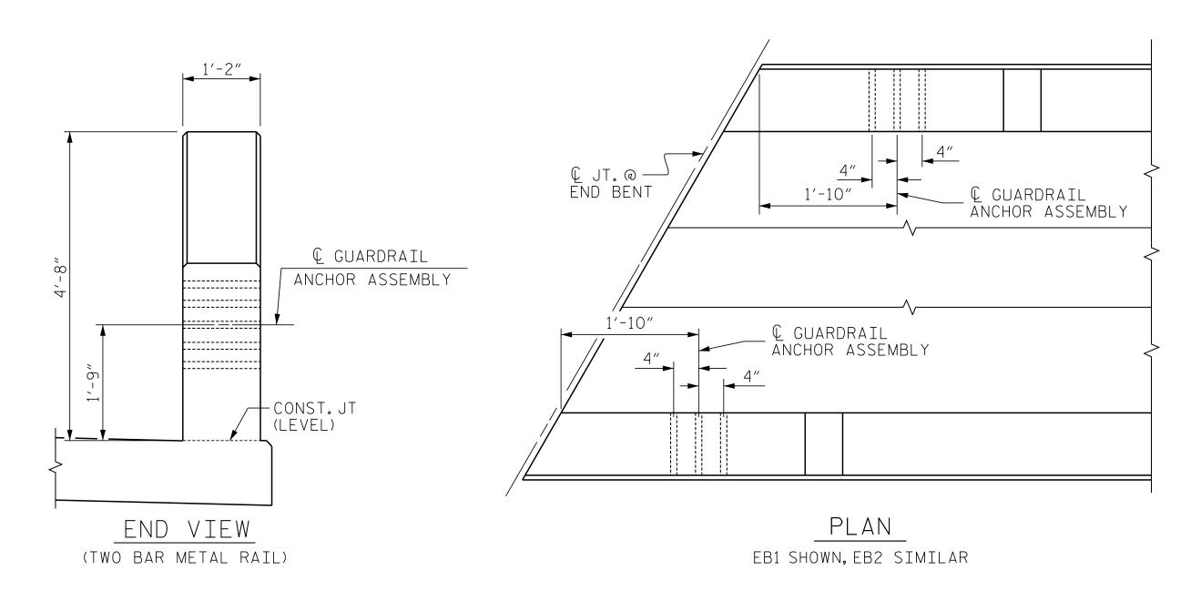
LOCATION OF GUARDRAIL ANCHOR AT END POST
