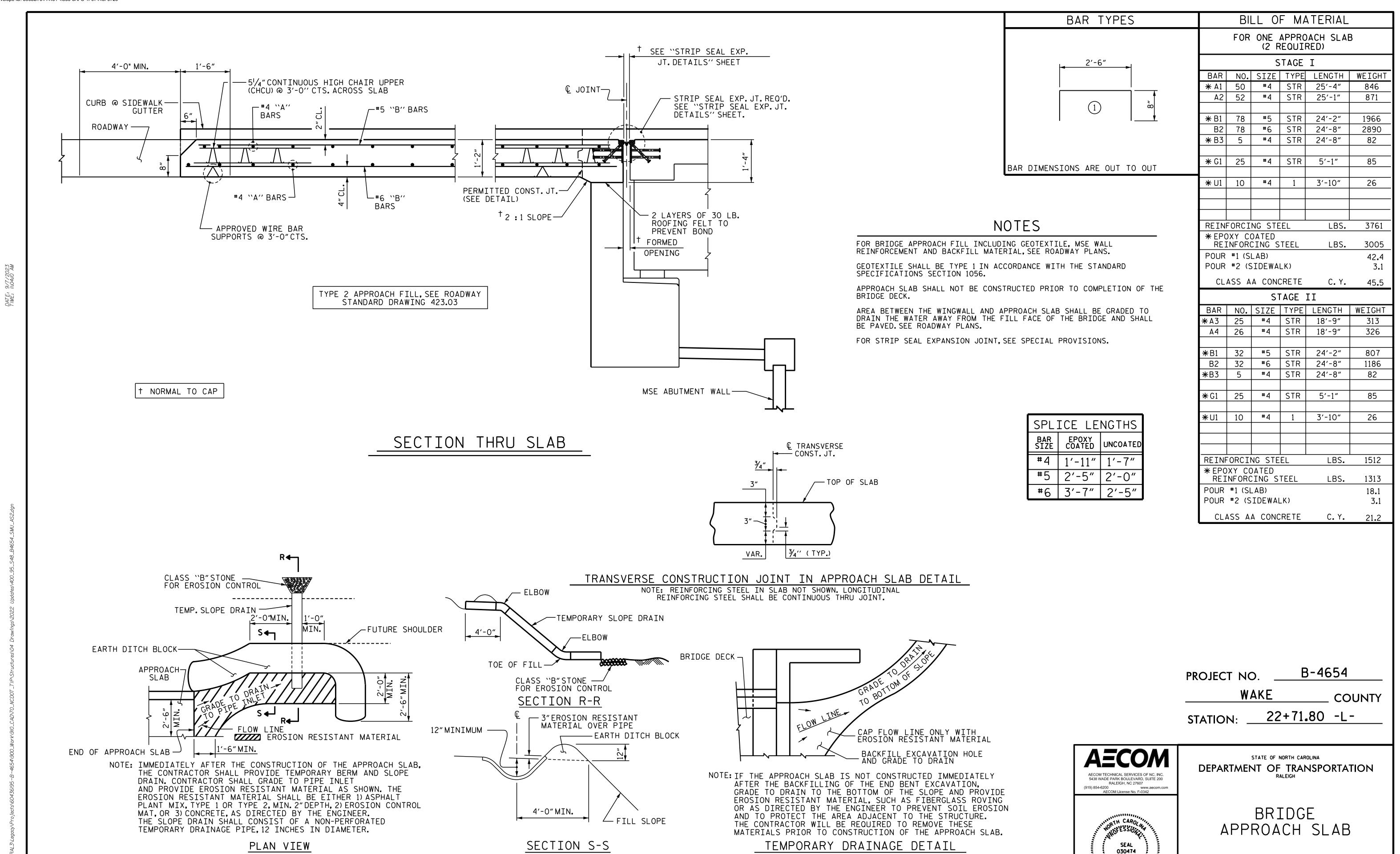
TEMPORARY BERM AND SLOPE DRAIN DETAILS
