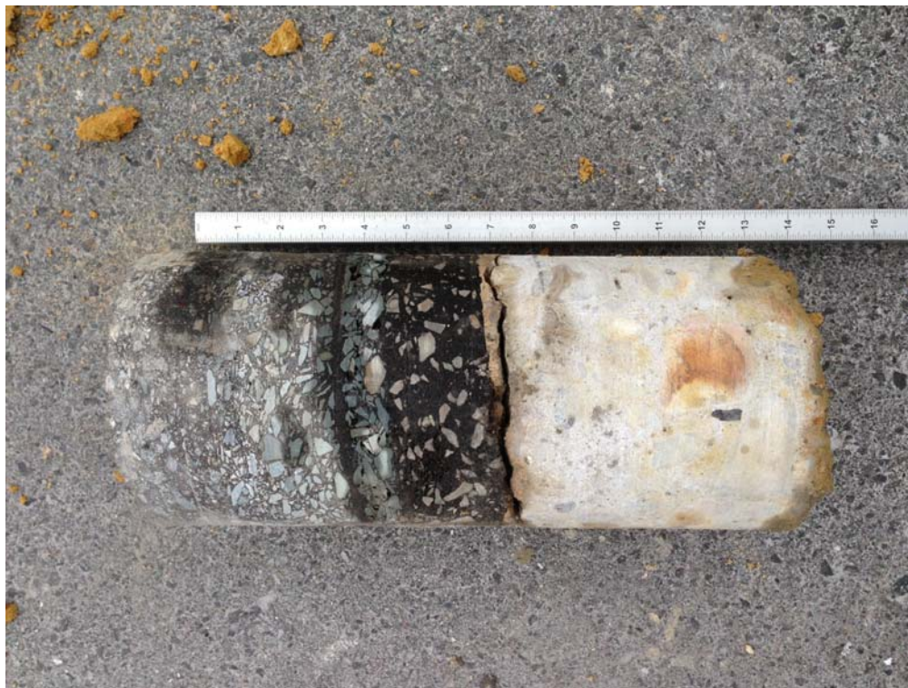
Exhibit A-21: Photograph of pavement core HA-03. Core HA-04 similar in condition and thickness.
