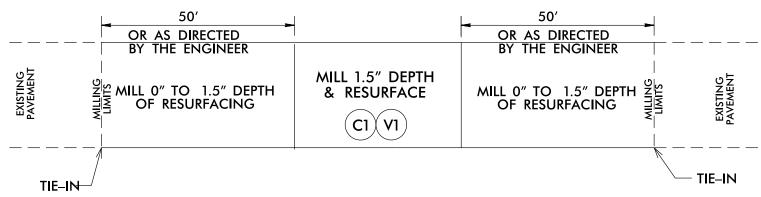
\* MILLING FOR APPROACHES SHALL BE PAID FOR UNDER INCIDENTAL MILLING
