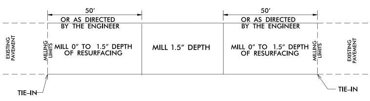
\* MILLING SHALL BE PAID FOR UNDER INCIDENTAL MILLING BRIDGE DRAWING FOR MAP #5 FORK CREEK MILL RD BRIDGE #384
