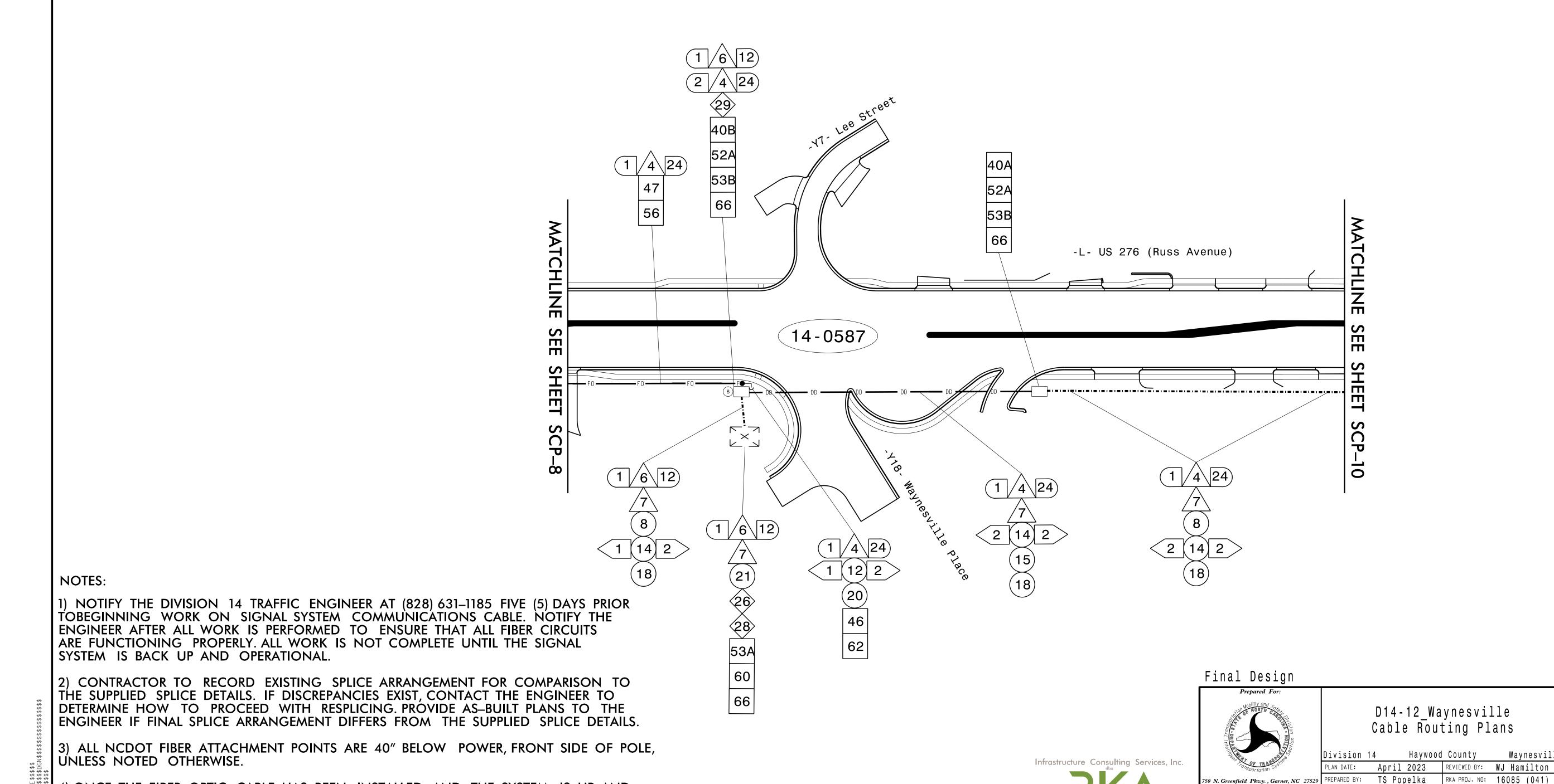
4) ONCE THE FIBER OPTIC CABLE HAS BEEN INSTALLED AND THE SYSTEM IS UP AND OPERATIONAL, REMOVE THE WIRELESS EQUIPMENT AND CONTACT THE DIVISION 14 TRAFFIC ENGINEER AT (828) 631–1185 AND RETURN THE WIRELESS EQUIPMENT.
