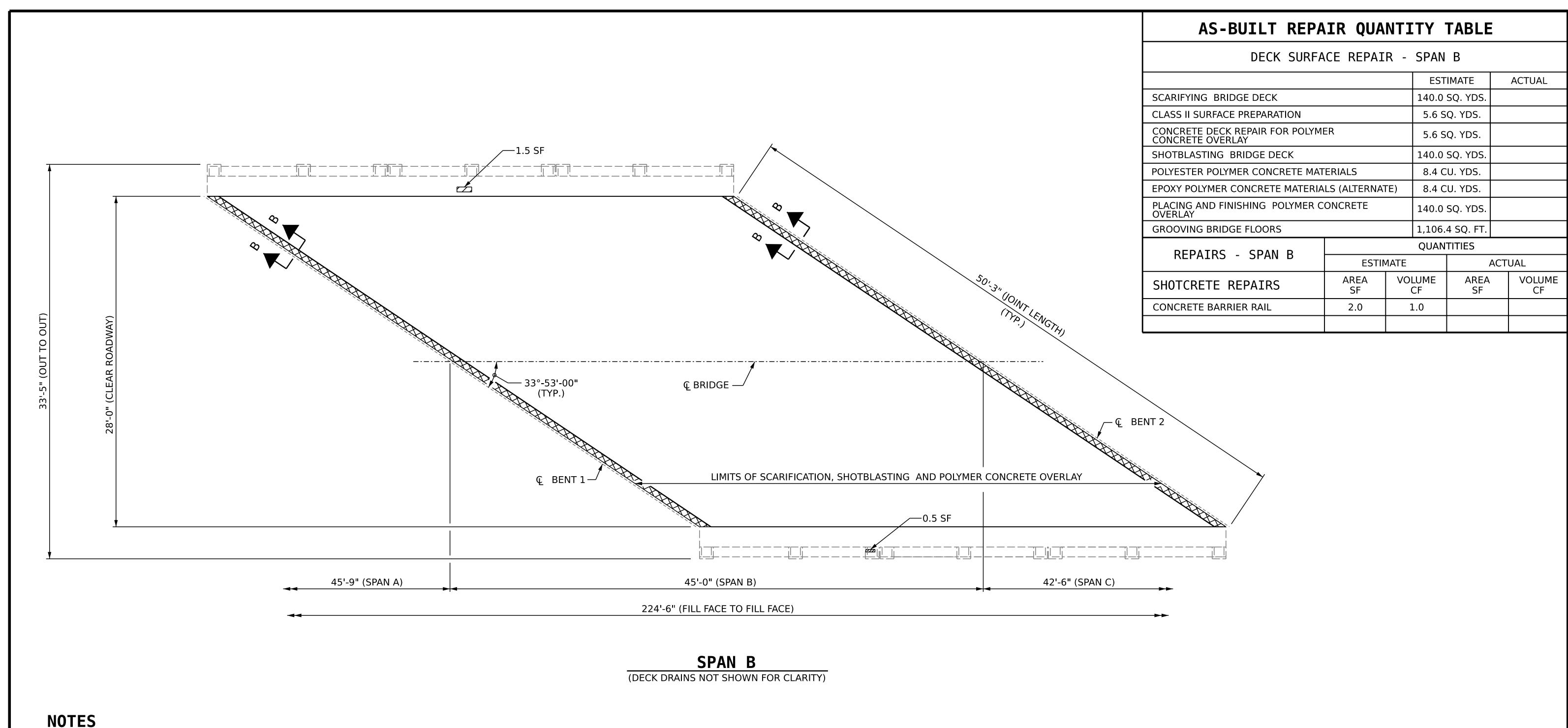
DECK SURFACE REPAIR QUANTITIES REPRESENT ESTIMATED VALUES OF CLASS II SURFACE PREPARATION AND CONCRETE DECK REPAIR FOR POLYMER CONCRETE OVERLAY AFTER REMOVAL OF UNSOUND CONCRETE (MIN. 2" CLEAR TO SAWCUT).
