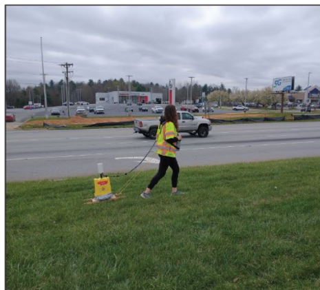
Photo 2. Collecting magnetometer data in Grid 1.
