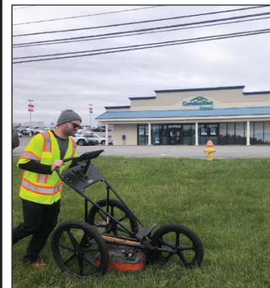
Photo 1. Collecting GPR data in Grid 1.
