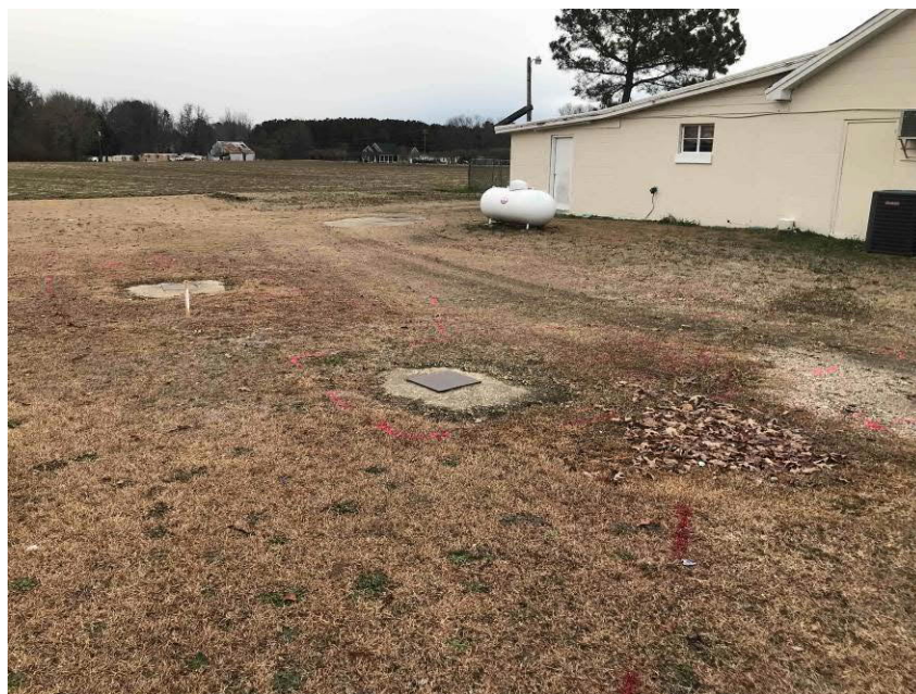
Photo #3 View of the two on-site probable USTs identified north of the on-site building in the geophysical investigation; facing northwest.
