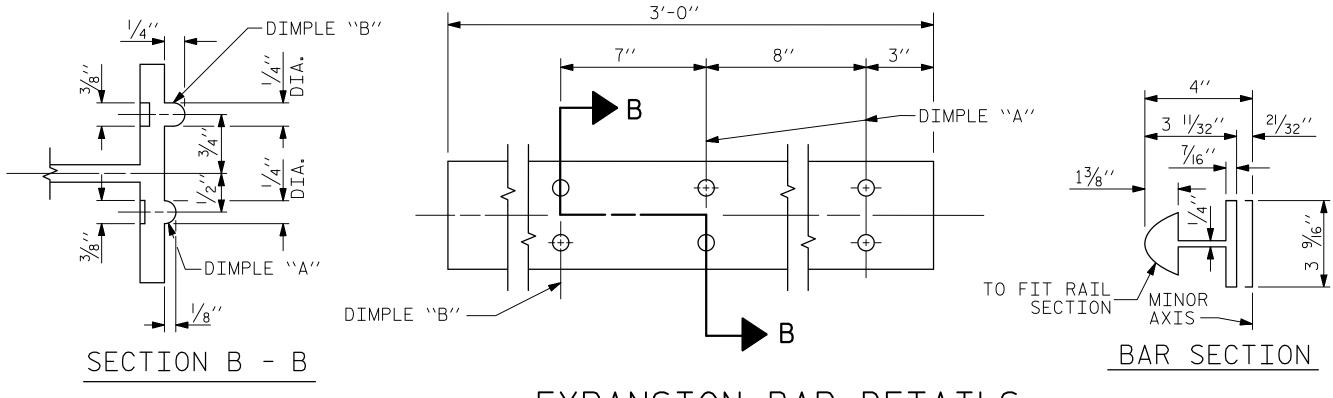
$/_2$ " Ø [13 THREAD] HOLE FOR  $/_2$ " Ø X 1" STAINLESS STEEL HEX HEAD CAP SCREW &  $1/_{16}$ " O.D.,  $1/_{32}$ " I.D.,  $/_{16}$ " THICK WASHER (TYP.)
