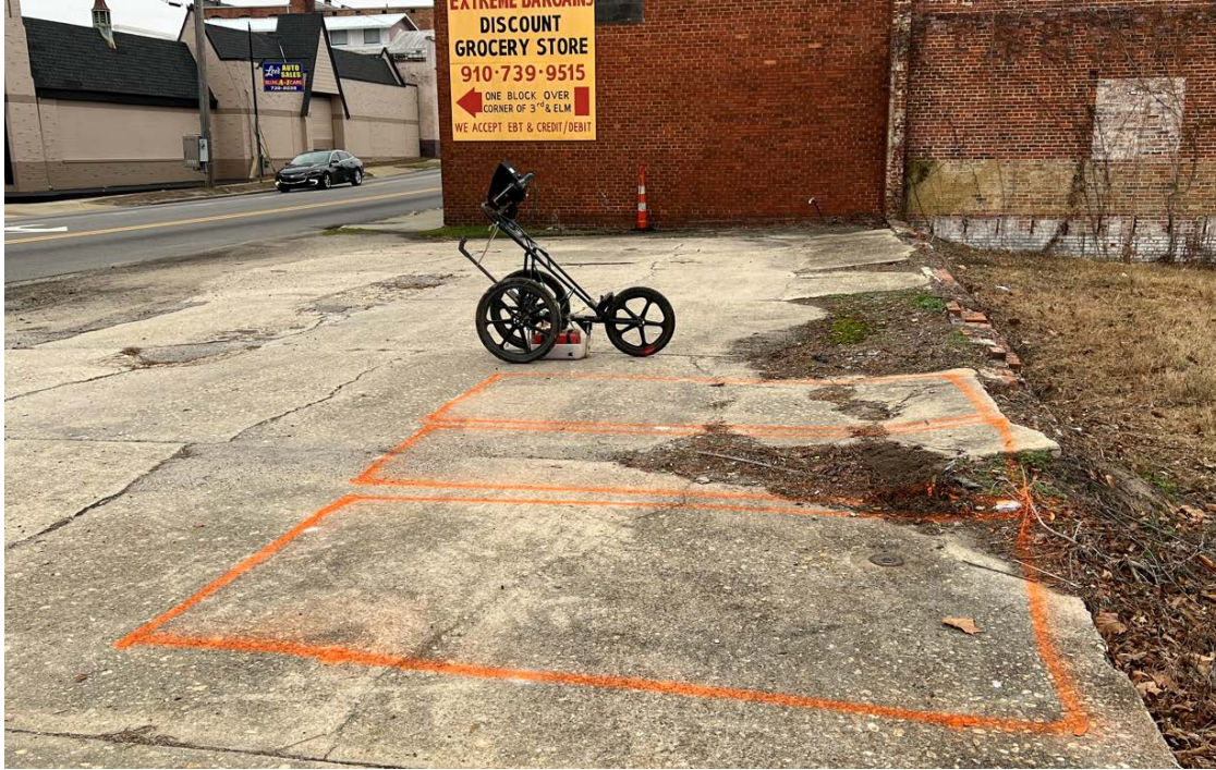
Photograph 1. Probable USTs identified with orange ground-marking paint.
