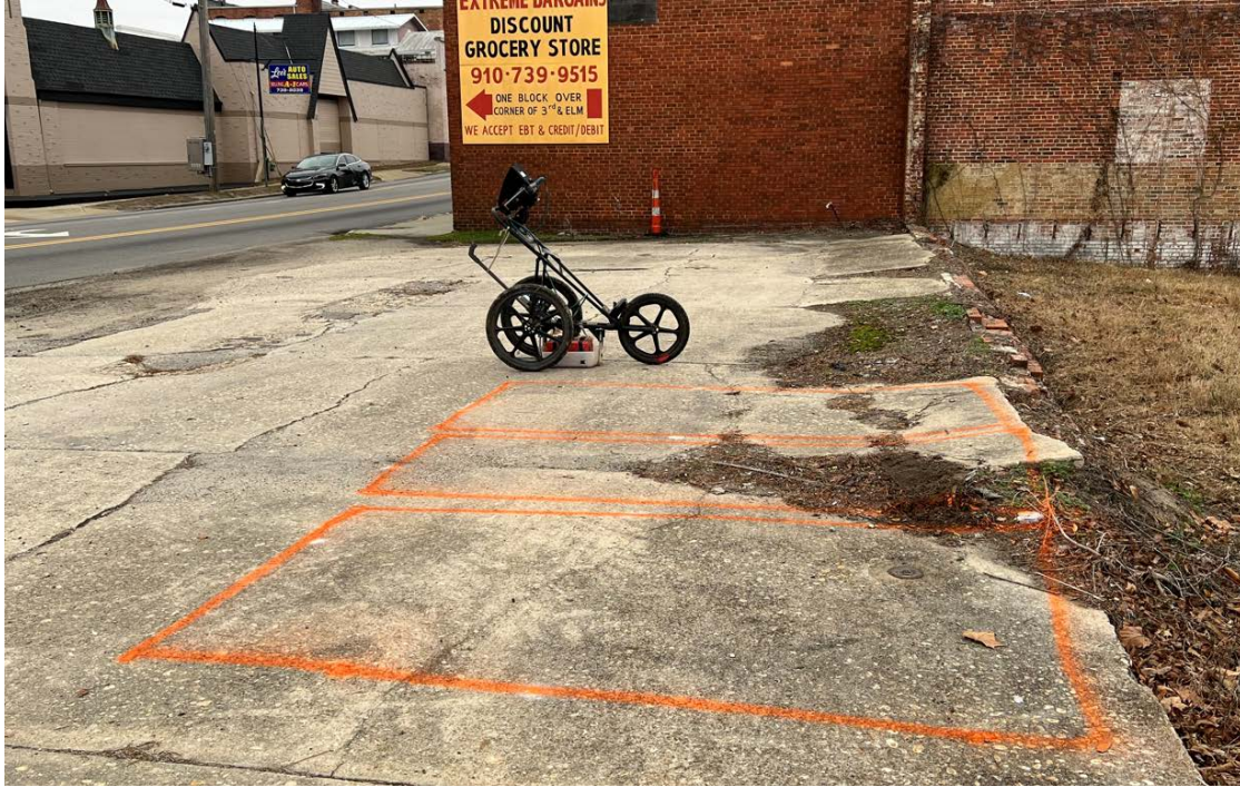
Photograph 1. Probable USTs identified with orange ground-marking paint.
