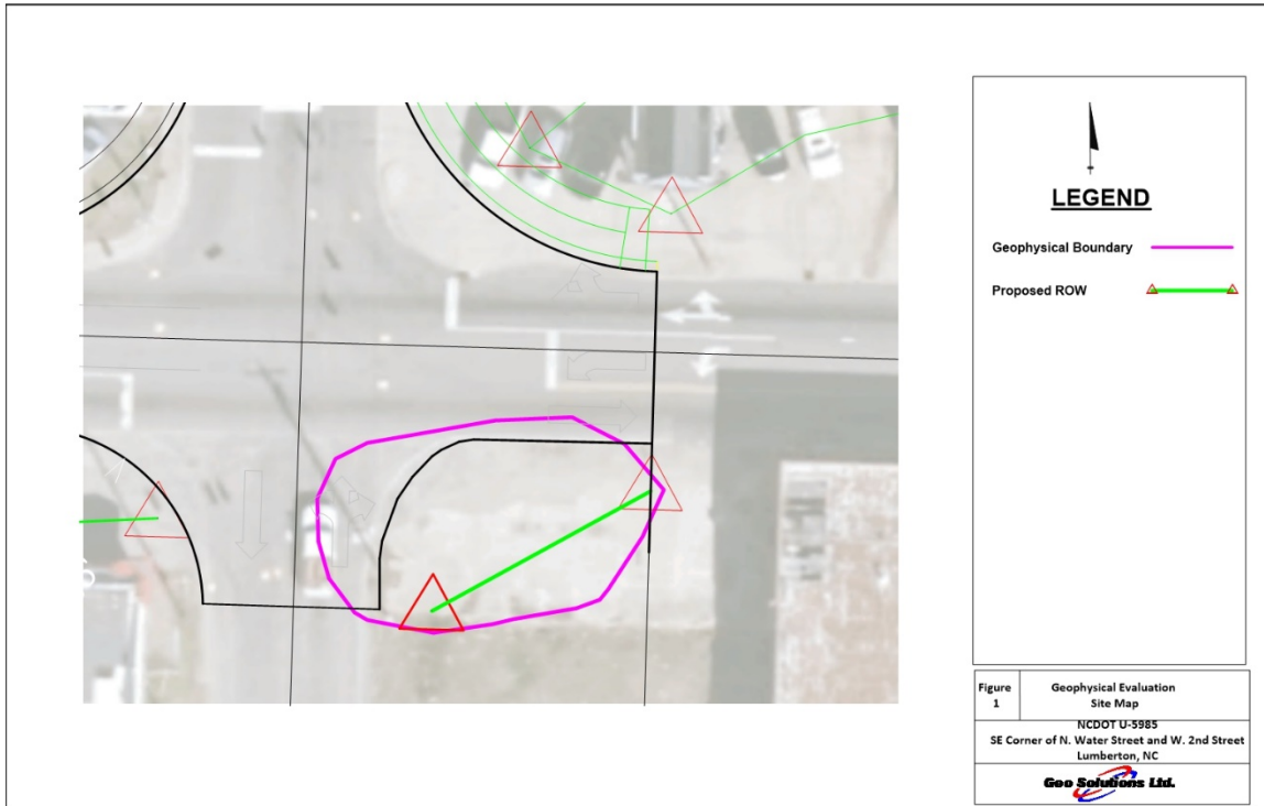
Figure 1. Site map of the area of the southeast corner of the NCDOT intersection widening project with the geophysical evaluation boundary delineated in magenta.
