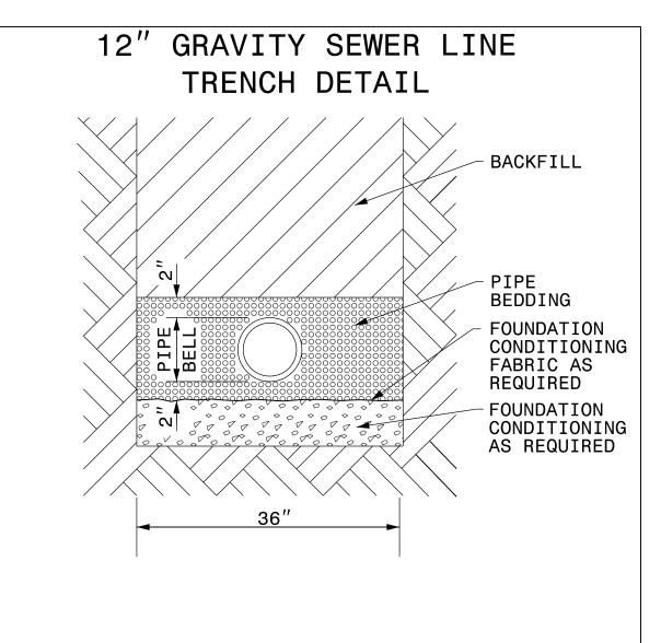
PLACE FOUNDATION CONDITIONING MATERIAL BELOW BEDDING IF REQUIRED, AS DIRECTED BY ENGINEER. PIPE BEDDED IN SELECT MATERIAL, CLASS II (TYPE 1) OR CLASS III. TRENCH BACKFILLED IN LOOSE 6" LAYERS COMPACTED TO TOP OF TRENCH USING LOCAL EXCAVATED MATERIAL IF APPROVED BY THE ENGINEER, OR SELECT MATERIAL. ALL MATERIAL SHALL BE FREE OF ROCKS, FOREIGN MATERIAL, AND FROZEN EARTH. COMPACTION SHALL BE TO APPROXIMATELY 95% DENSITY IN ACCORDANCE WITH AASHTO T-99 AS MODIFIED BY THE DEPARTMENT OF TRANSPORTATION.
