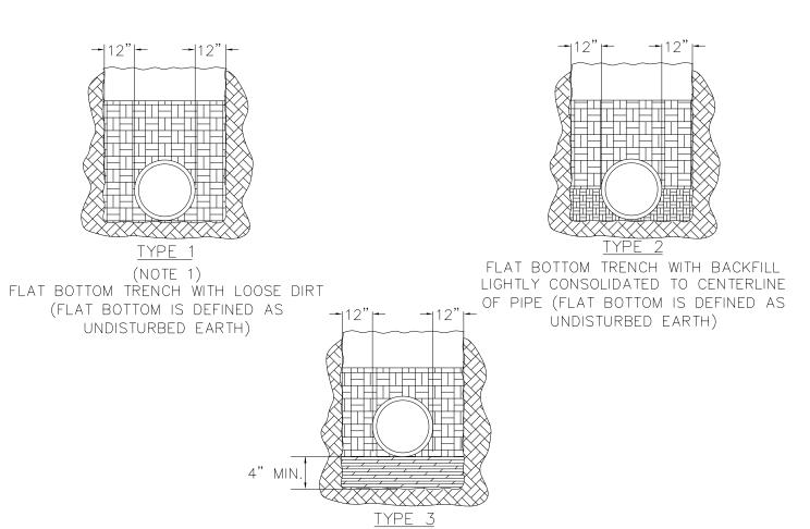
PIPE BEDDED IN 4" MINIMUM LOOSE SOIL WITH BACKFILL LIGHTLY CONSOLIDATED TO TOP OF PIPE (LOOSE SOIL IS DEFINED AS NATIVE SOIL EXCAVATED FROM THE TRENCH, FREE OF ROCK, ORGANIC MATERIAL, FOREIGN MATERIALS AND FROZEN EARTH.)
