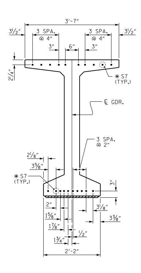
DETAIL "C" \*NOTE: S7 BARS SHALL BE BENT BEFORE SHIPMENT. HEAT BENDING SHALL NOT BE ALLOWED.
