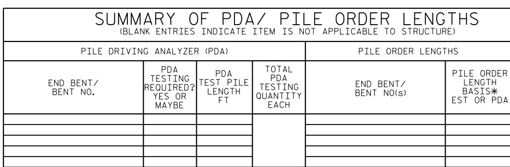
\* EST=PILE ORDER LENGTHS FROM ESTIMATED PILE LENGTHS; PDA=PILE ORDER LENGTHS BASED ON PDA TESTING. FOR GROUPS OF END BENTS/BENTS WITH PILE ORDER LENGTHS BASED ON PDA TESTING, THE FIRST END BENT/ BENT NO.LISTED FOR EACH GROUP IS THE REPRESENTATIVE END BENT/ BENT WITH THE PDA.
