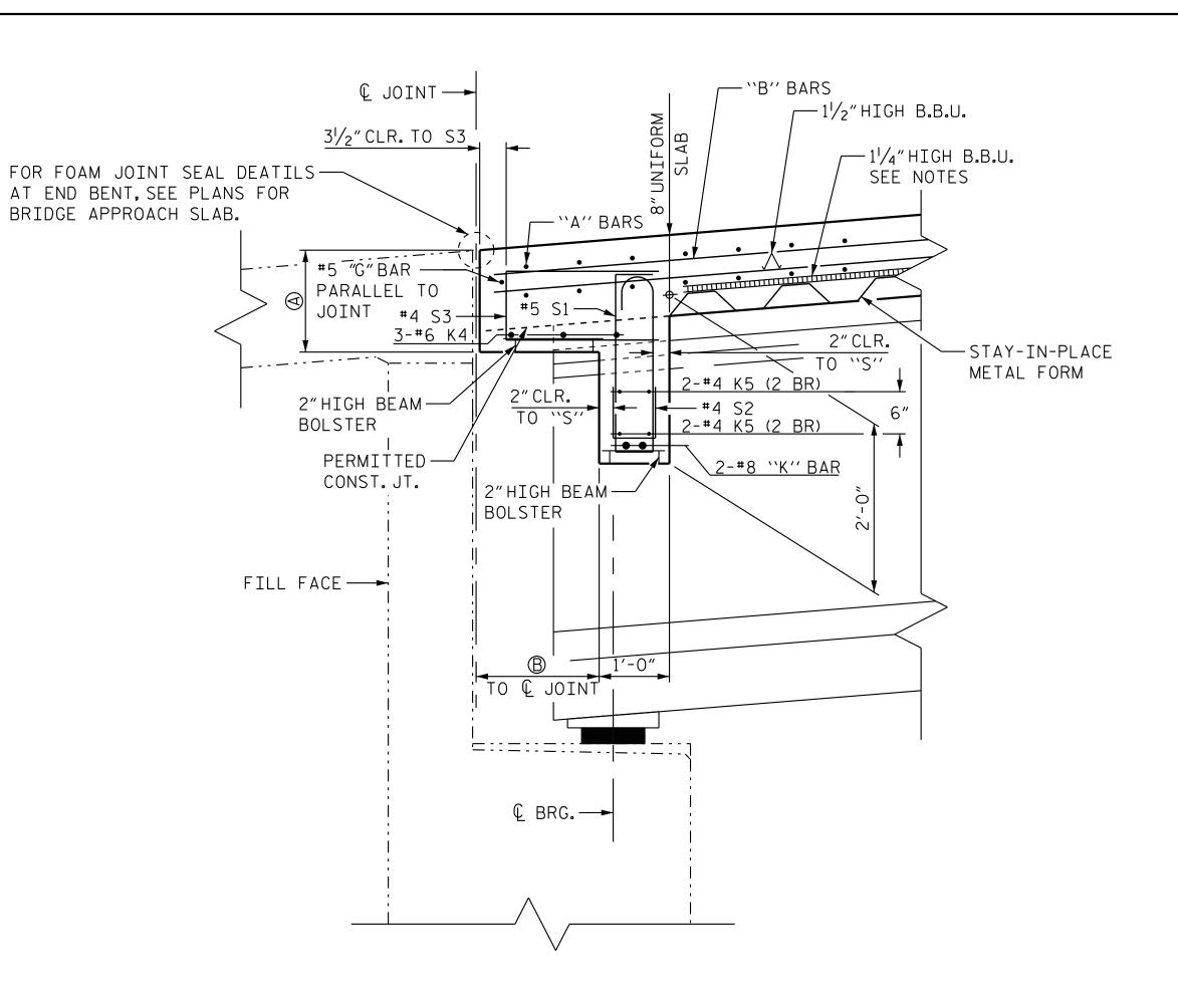
(A): 1'-2"@ END BENT 1; 1'-3 $\frac{1}{2}$ "@ END BENT 2 (B): 1'-10"@ END BENT 1; 1'-10"@ END BENT 2
