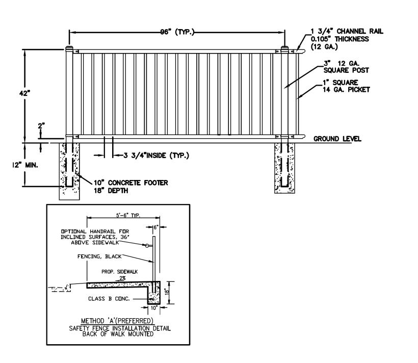
2. BOTTOM OF POSTS TO BE EMBEDDED IN CONCRETE SHOULD FIRST BE PROTECTED WITH TWO—PART EPOXY DIPPING OR ZINC CHROMATE COATING TO PREVENT CORROSION.
