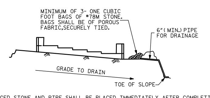
BAGGED STONE AND PIPE SHALL BE PLACED IMMEDIATELY AFTER COMPLETION OF END BENT EXCAVATION. PIPE MAY BE EITHER CONCRETE, CORRUGATED STEEL, CORRUGATED ALUMINUM ALLOY, OR CORRUGATED PLASTIC. PERFORATED PIPE WILL NOT BE ALLOWED.
