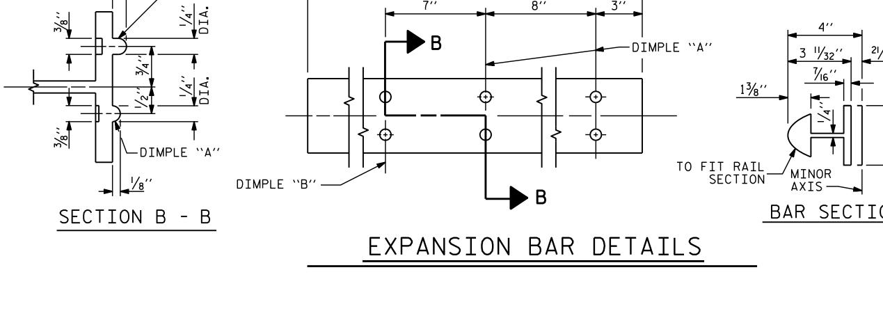
1/2" Ø [13 THREAD] HOLE FOR 1/2" Ø X 1" STAINLESS STEEL HEX HEAD CAP SCREW & 1/16" O.D., 17/32" I.D., — 1/16" THICK WASHER (TYP.)
