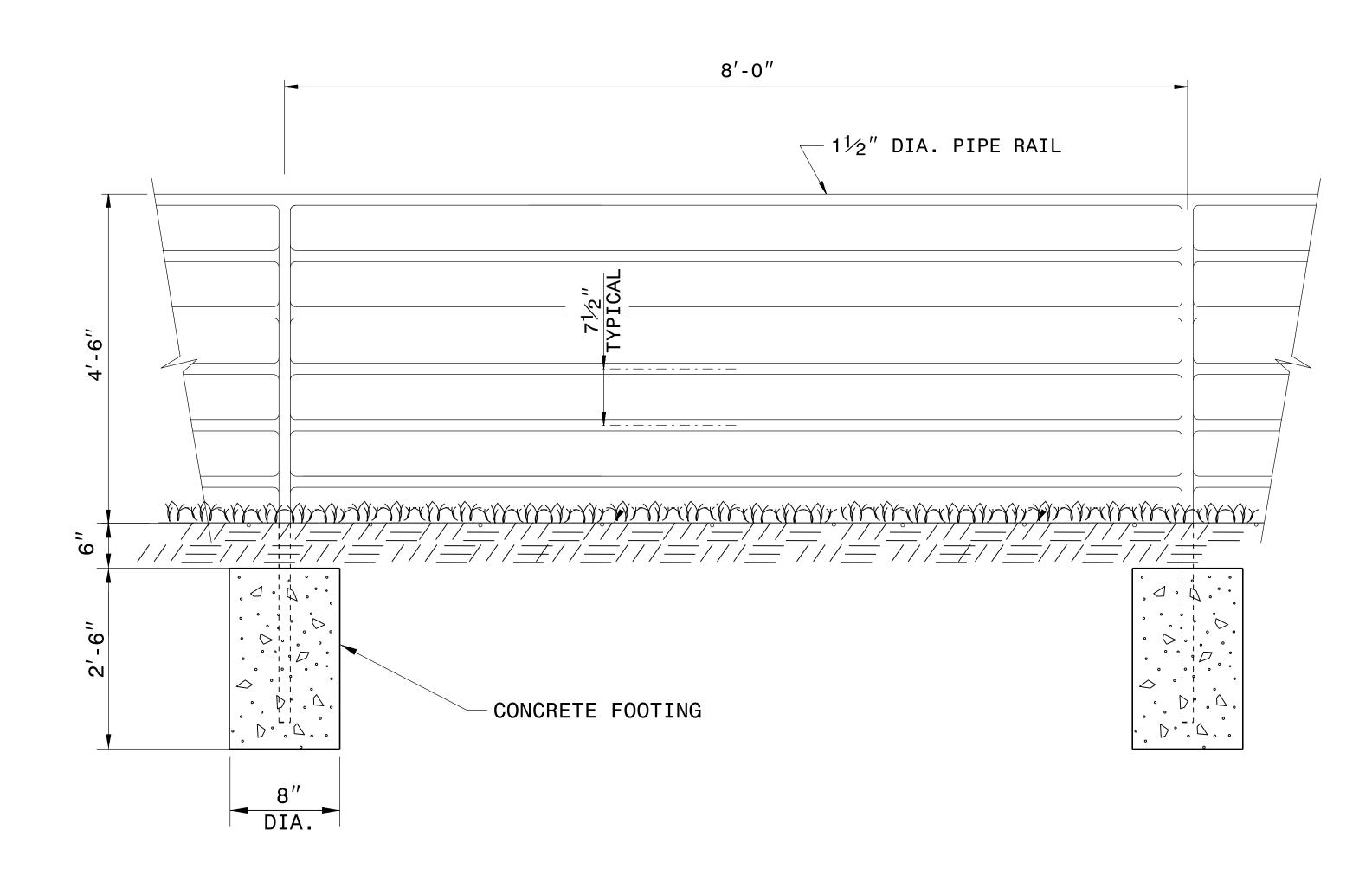
**ELEVATION OF HANDRAIL**
