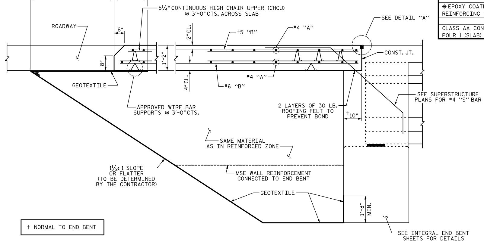
SECTION THRU SLAB (TYPE III APPROACH FILL)
