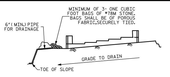
BAGGED STONE AND PIPE SHALL BE PLACED IMMEDIATELY AFTER COMPLETION OF END BENT EXCAVATION. PIPE MAY BE EITHER CONCRETE, CORRUGATED STEEL, CORRUGATED ALUMINUM ALLOY, OR CORRUGATED PLASTIC. PERFORATED PIPE WILL NOT BE ALLOWED.
