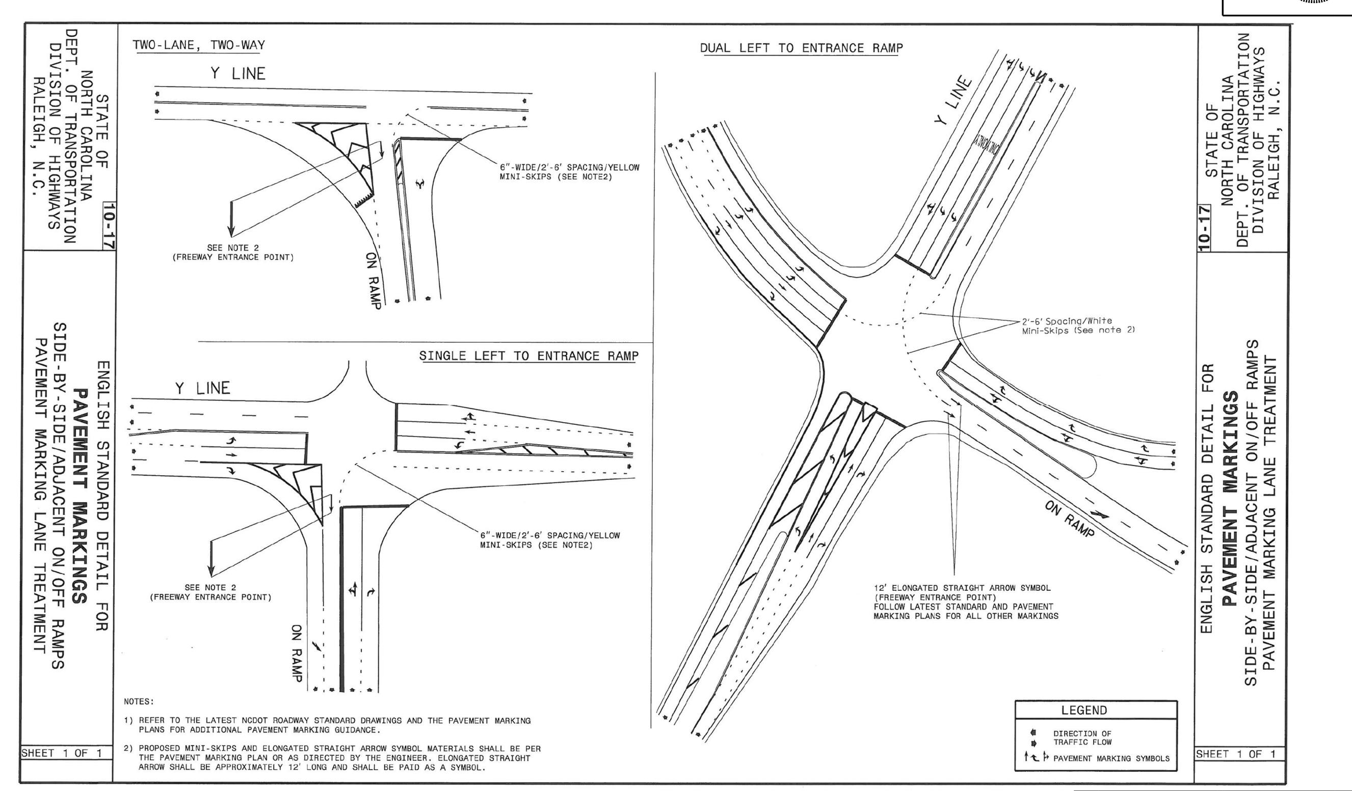
REVISED PAVEMENT MARKING ROADWAY STANDARD DRAWING
