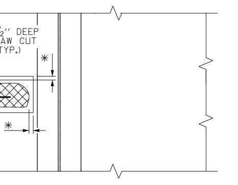
\* REMOVE CONCRETE UNTIL SOUND CONCRETE IS FOUND (1''MIN.DEPTH)
