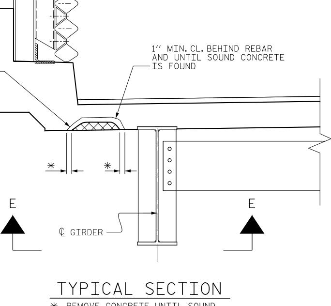
\* REMOVE CONCRETE UNTIL SOUND CONCRETE IS FOUND (1" MIN.DEPTH)
