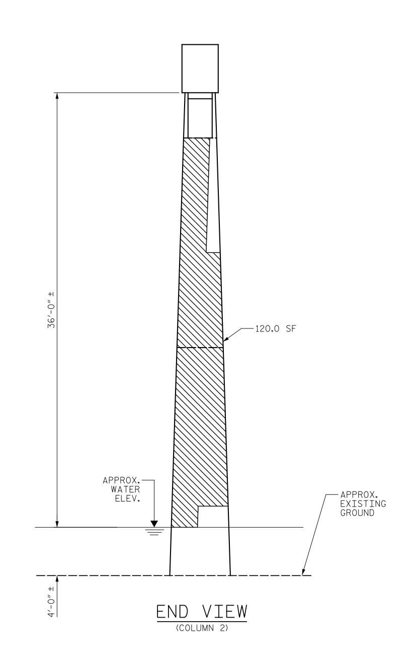
AS-BUILT REPAIR QUANTITY TABLE QUANTITIES BENT 4 REPAIRS ESTIMATE ACTUAL AREA DEPTH VOLUME AREA VOLUME SHOTCRETE REPAIRS FΤ CAP 0.0 0.0 COLUMN 421.1 210.6 STRUT 36.1 18.1 CONCRETE REPAIRS 0.0 LENGTH LENGTH EPOXY RESIN INJECTION CAP 0.0 COLUMN 0.0 STRUT 0.0 SQ. SQ. FT EPOXY COATING TOP OF BENT CAP 103
