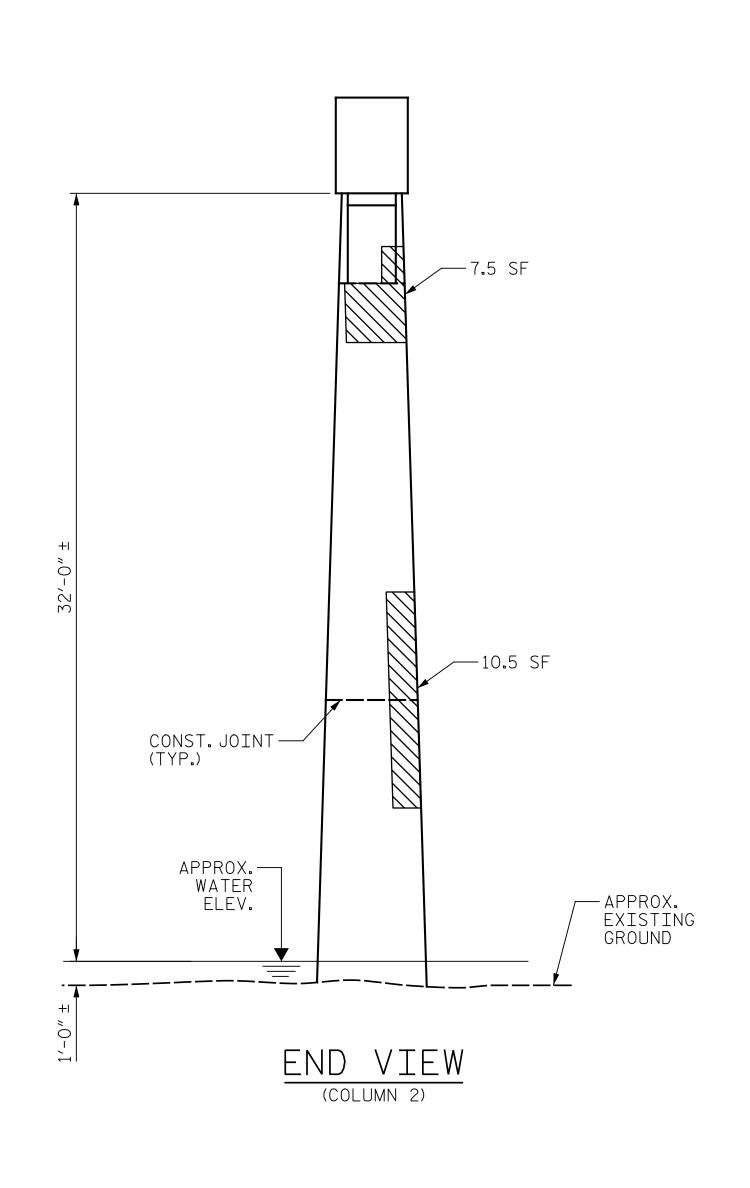
QUANTITIES BENT 6 REPAIRS ESTIMATE ACTUAL AREA | DEPTH | VOLUME AREA VOLUME SHOTCRETE REPAIRS SF CF FΤ CF 0.0 0.0 52.0 26.0 COLUMN STRUT 5.7 11.4 CONCRETE REPAIRS 0.0 LENGTH LENGTH EPOXY RESIN INJECTION LF CAP 0.0 COLUMN 0.0 STRUT 0.0 SQ. FT SQ. FT EPOXY COATING TOP OF BENT CAP 103
