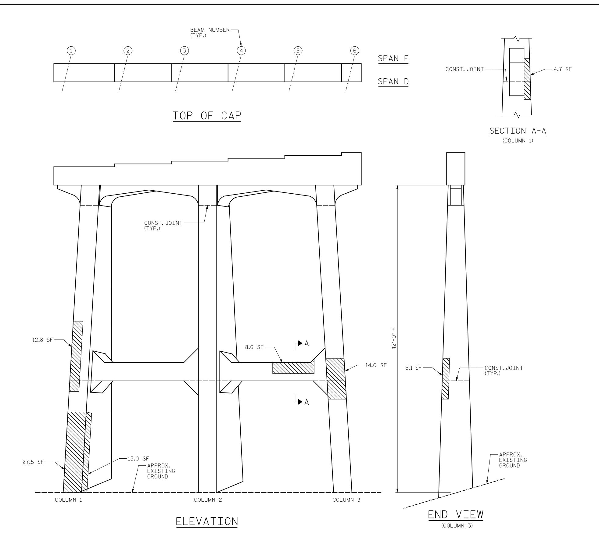
AS-BUILT REPAIR QUANTITY TABLE QUANTITIES BENT 4 REPAIRS ESTIMATE ACTUAL AREA DEPTH VOLUME VOLUME AREA SHOTCRETE REPAIRS SF CF FΤ CF CAP 9.0 4.5 COLUMN 157.1 78.6 STRUT 27.0 13.5 CONCRETE REPAIRS 0.0 LENGTH LENGTH EPOXY RESIN INJECTION LF CAP 0.0 COLUMN 0.0 STRUT 0.0 SQ. FT SQ. FT EPOXY COATING TOP OF BENT CAP
