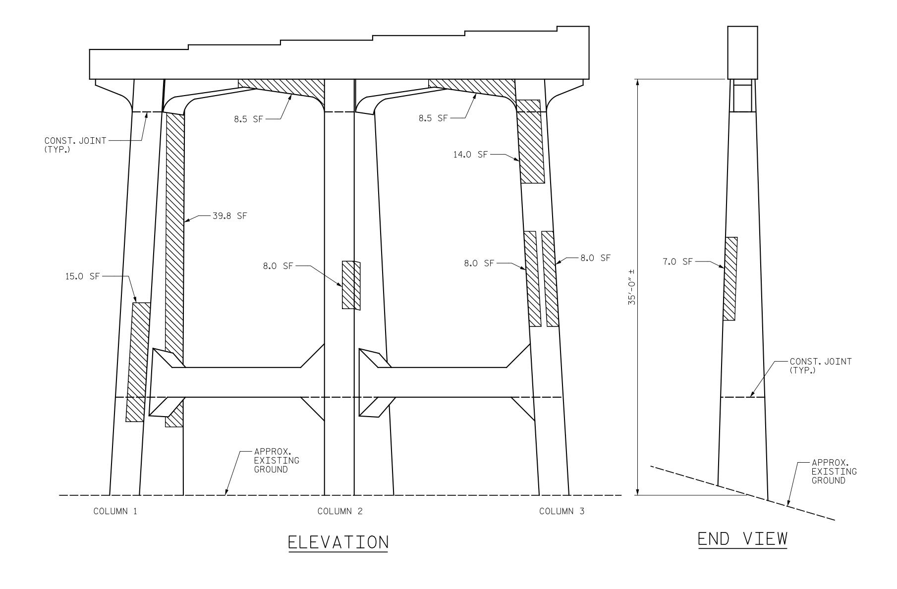
AS-BUILT REPAIR QUANTITY TABLE QUANTITIES BENT 1 REPAIRS ESTIMATE ACTUAL AREA | DEPTH | VOLUME AREA VOLUME SHOTCRETE REPAIRS SF CF FΤ CF CAP 31.6 15.8 COLUMN 249.4 124.7 STRUT 47.1 23.6 CONCRETE REPAIRS 0.0 LENGTH LENGTH EPOXY RESIN INJECTION LF 0.0 COLUMN 0.0 STRUT 0.0
