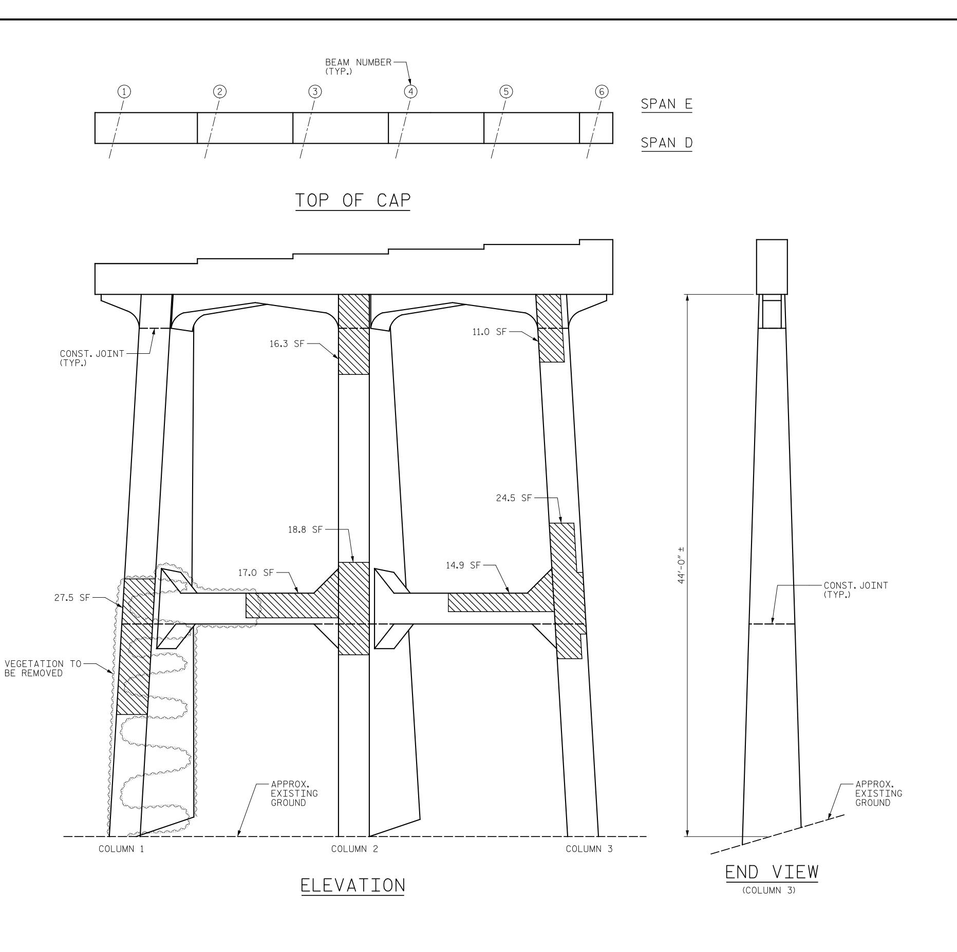
AS-BUILT REPAIR QUANTITY TABLE QUANTITIES BENT 4 REPAIRS ESTIMATE ACTUAL AREA | DEPTH | VOLUME AREA VOLUME SHOTCRETE REPAIRS SF CF FΤ CF CAP 0.0 0.0 COLUMN 127.9 64.0 STRUT 107.3 53.7 CONCRETE REPAIRS 0.0 LENGTH LENGTH EPOXY RESIN INJECTION LF 0.0 COLUMN 0.0 STRUT 0.0 SQ. FT SQ. FT EPOXY COATING TOP OF BENT CAP 91
