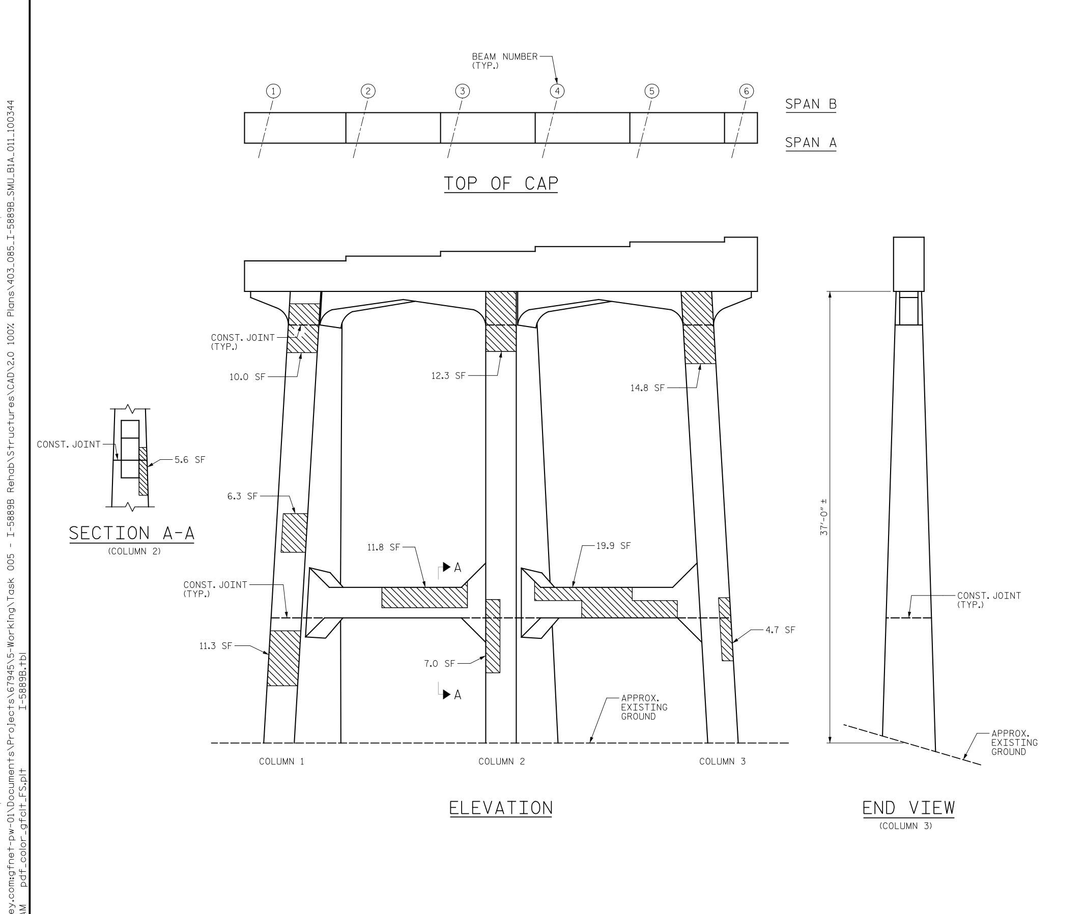
AS-BUILT REPAIR QUANTITY TABLE QUANTITIES BENT 1 REPAIRS ESTIMATE ACTUAL AREA DEPTH VOLUME AREA VOLUME SHOTCRETE REPAIRS SF CF CF FΤ 0.0 0.0 COLUMN 232.3 116.2 STRUT 72.5 36.3 CONCRETE REPAIRS 0.0 LENGTH LENGTH EPOXY RESIN INJECTION LF CAP 0.0 COLUMN 0.0 STRUT 0.0 SQ. FT SQ. FT
