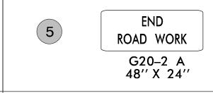
PLACE 500' FOLLOWING THE END OF CONSTRUCTION LIMITS OR AS SHOWN WHEN WORK ENDS AT A 3-WAY TEE INTERSECTION.
