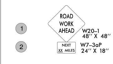
PLACE 1000' PRIOR TO BEGINNING OF CONSTRUCTION LIMITS. ONLY USED ON -Y- LINES IF RESURFACING LIMITS EXTEND 1000' ALONG -Y- LINE.
