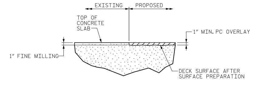
DETAIL OF POLYMER CONCRETE OVERLAY
