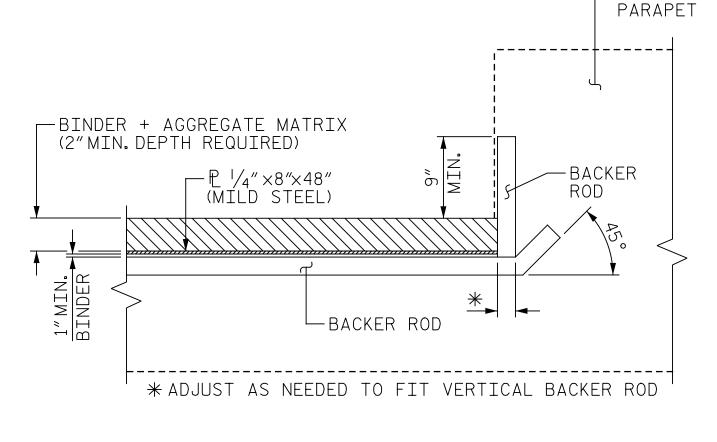
SECTION H-H (PROPOSED JOINT SEAL)
